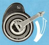
Smooth crank-action handle advances film, cocks the shutter, counts exposures and prevents double exposures—all automatically. The window guide is your check on whether 12 or 24 exposure film is being used.
